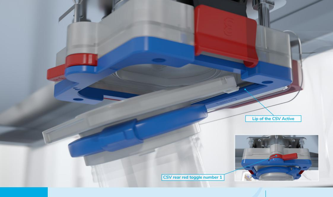
To dock the chargebag, slide the front of the passive connection under the lip of the CSV Active, then push the passive connection flat and fully turn the CSV's rear red toggle, marked 1, to release the interlocks.
