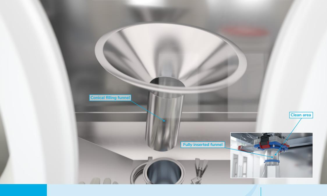
Now insert the Ezi-Flow conical filling funnel, ensuring the funnel is fully inserted through the filling band into the chargebag. Ensure the filling band is positioned towards the end of the funnel to maintain a clean area during the filling process.
