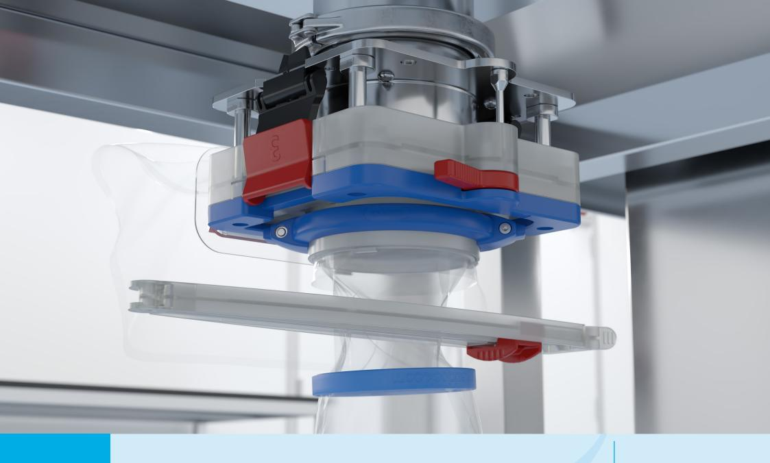
Raise the two red side toggles marked number 3, push in the red handle marked number 2 and finally turn the rear red toggle, marked 1. Care should be taken not to allow the chargebag to fall when this final toggle is turned.
