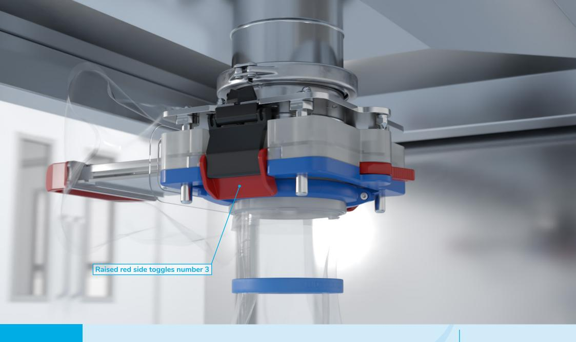
At this point there is a void in the system, and so the two red side toggles marked number 3 need to be fully raised. This lowers the active cassette onto the active spigot and creates a contained seal.
