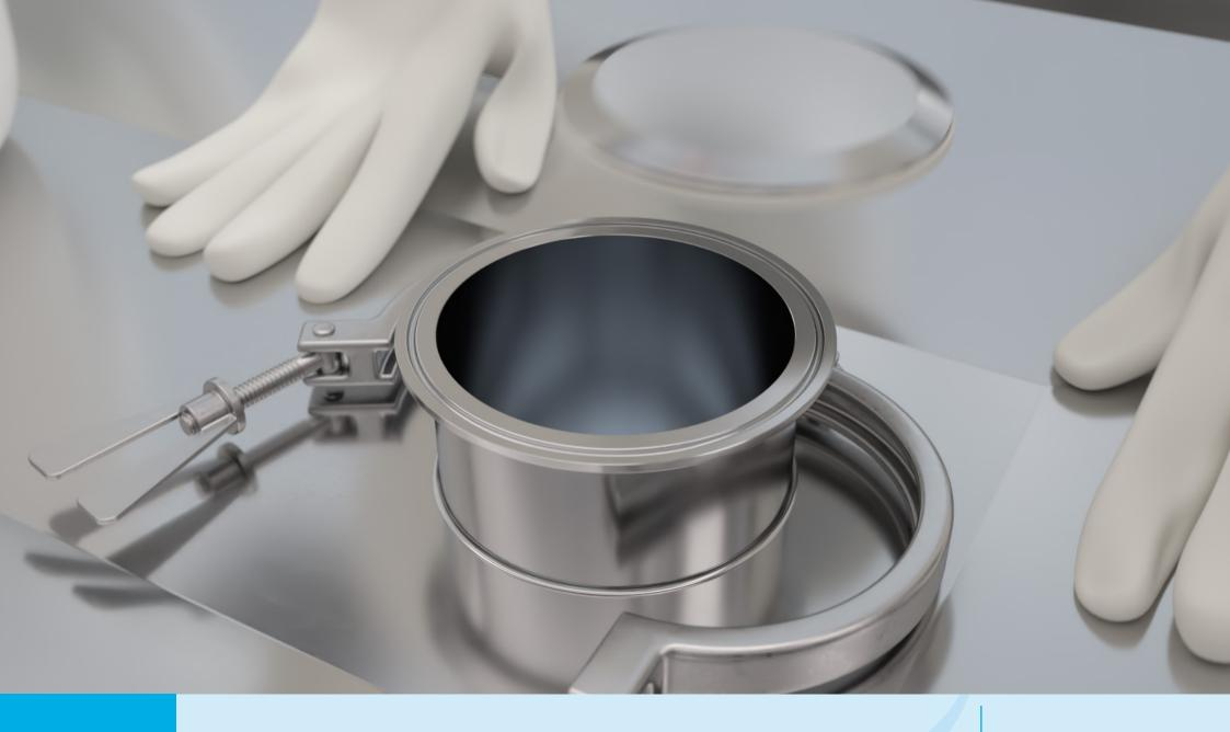
Working within the isolator, first remove the blanking cap which covers the transfer chute.
