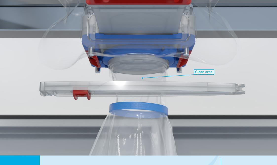
Before removing the chargebag, first use the Ezi-Grip Single-use bag clamp to seal off the neck of the chargebag. Be sure to position the clamp in the clean area, between the passive and the filling band.
