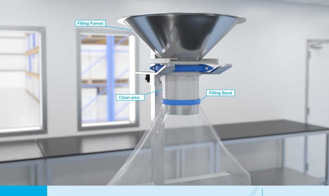
Fully insert the Filling Funnel through the Passive Body. The Filling Band must tightly wrap around the Filling Funnel and should be positioned towards the end of the Funnel Spout. This will create a "Clean Area" and prevent product from contaminating the Chargebag Neck & Passive during the Filling Process.
