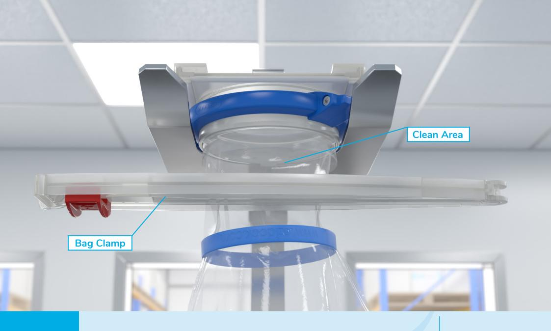
Next, the Ezi-Grip Single-Use Bag Clamp needs to be used to seal off the neck of the Chargebag and prevent product from contaminating the Passive. Be sure to position the Clamp in the "Clean Area" between the Passive and the Filling Band.
