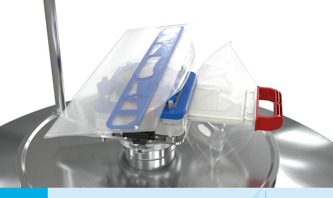
Before removing the chargebag, first manipulate it to ensure any residual materials are fully discharged. Then, fold down the chargebag prior to removal. You then simply reverse the docking process.
