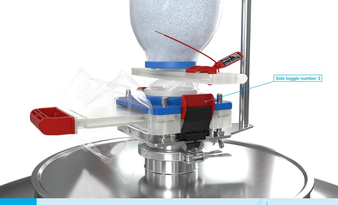
The removal of the sliders has left a void in the system, which the next operation deals with. Fully raising the two red side toggles, marked number 3, removes this void, by lowering the active cassette onto the active spigot and creating a contained seal.
