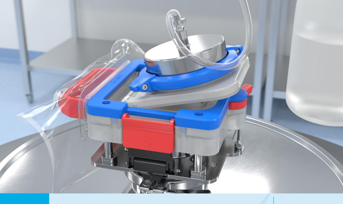
Insert the front of the passive under the lip of the active, as pictured, and push down flat at the rear.
