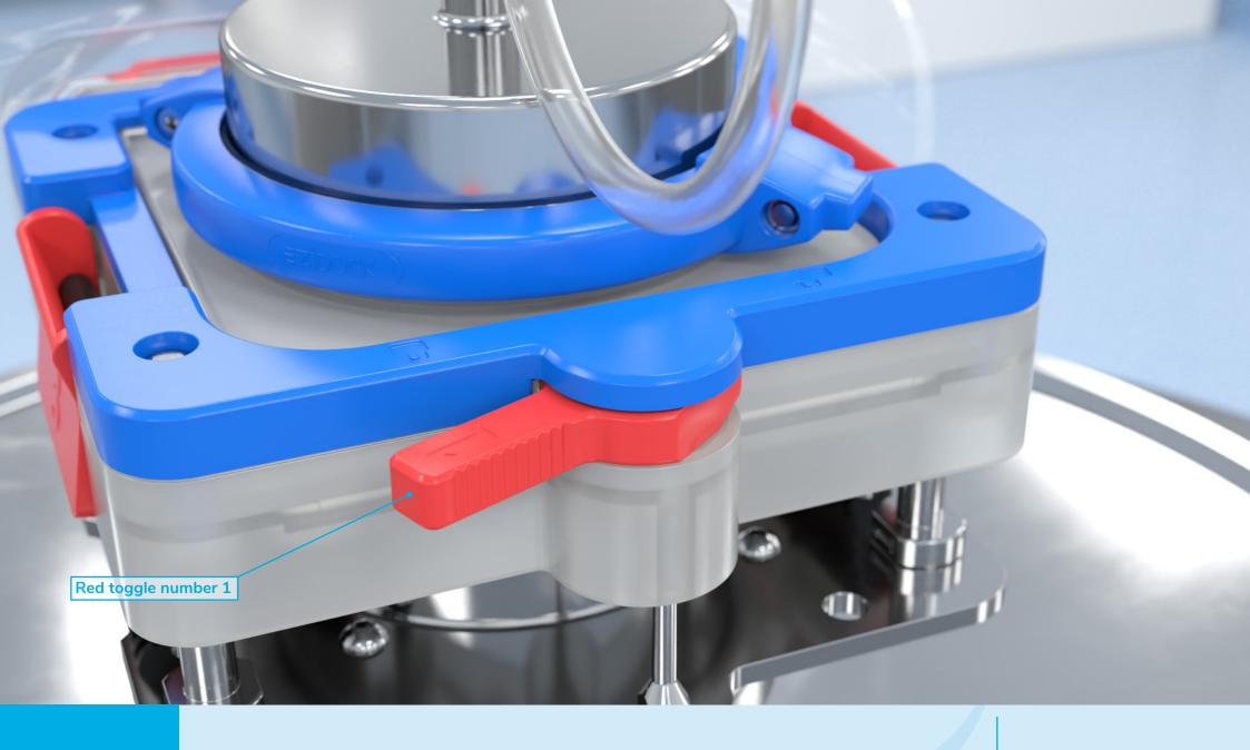
Now you can fully turn the rear toggle, marked number 1, to release the interlocks.
