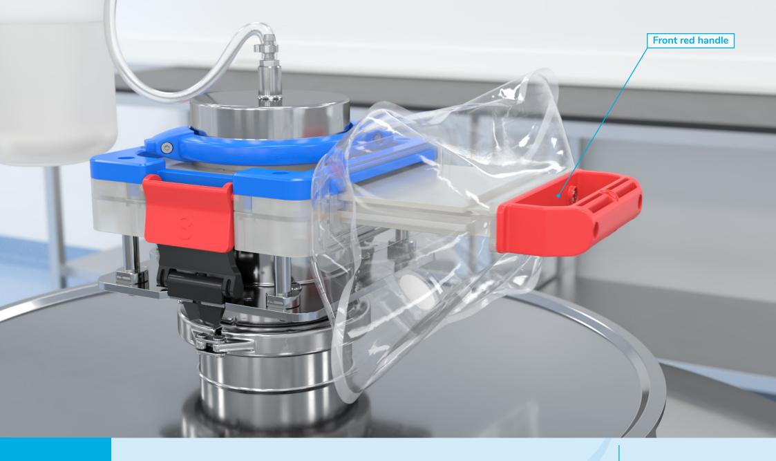
Next, pull out the front red handle marked number 2. This removes the active and passive sliders.
