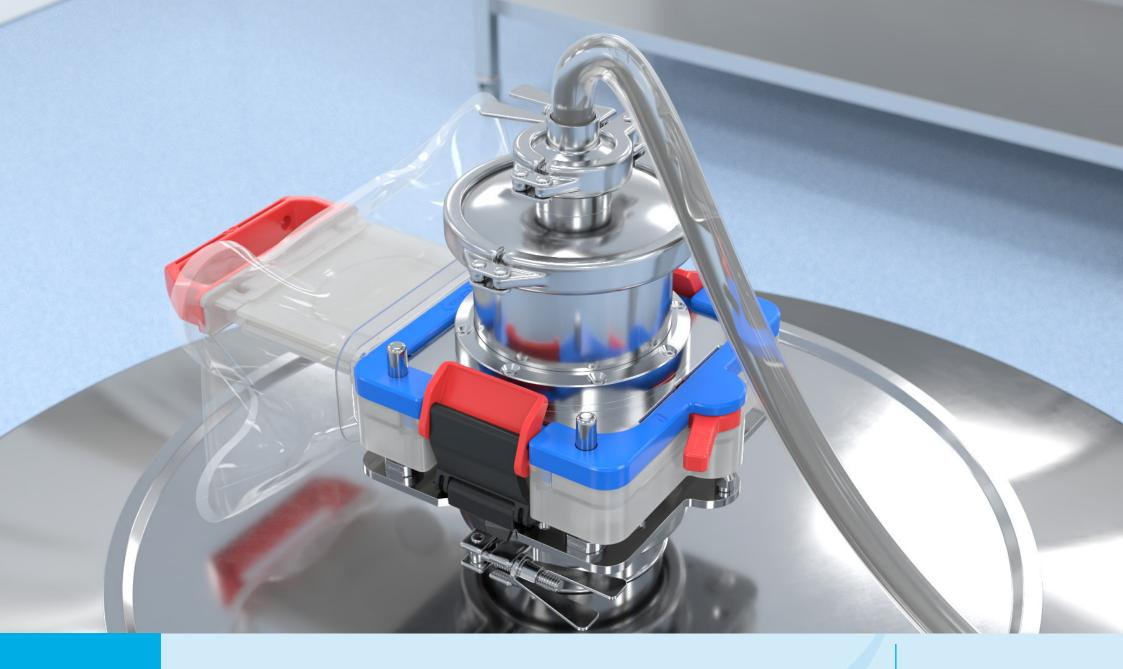
The Active can now be washed down by releasing the cleaning fluid through the sprayball
