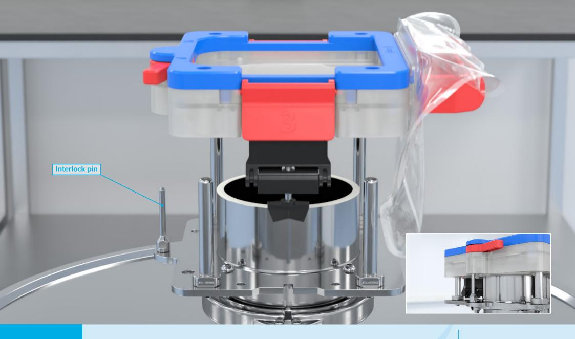
Ensure that the interlock pin is at the rear.
