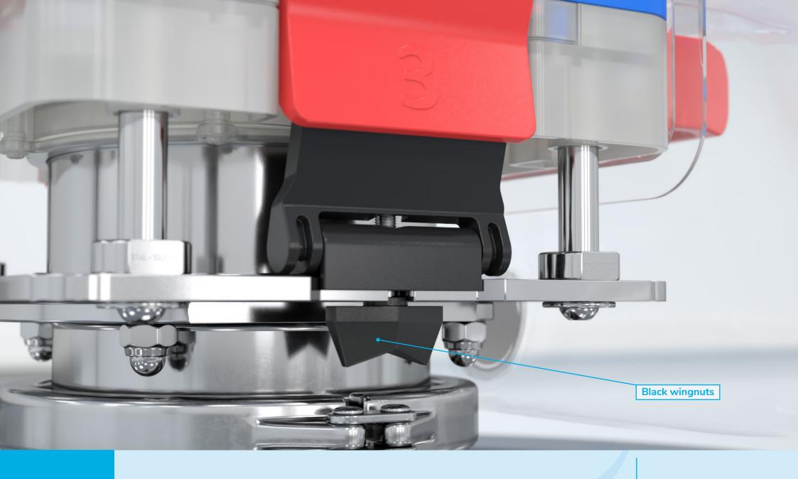
Now that the internal surfaces are washed down, you can remove the cassette as follows: First, loosen the black wingnuts, which are located under the red number 3 side toggles.
