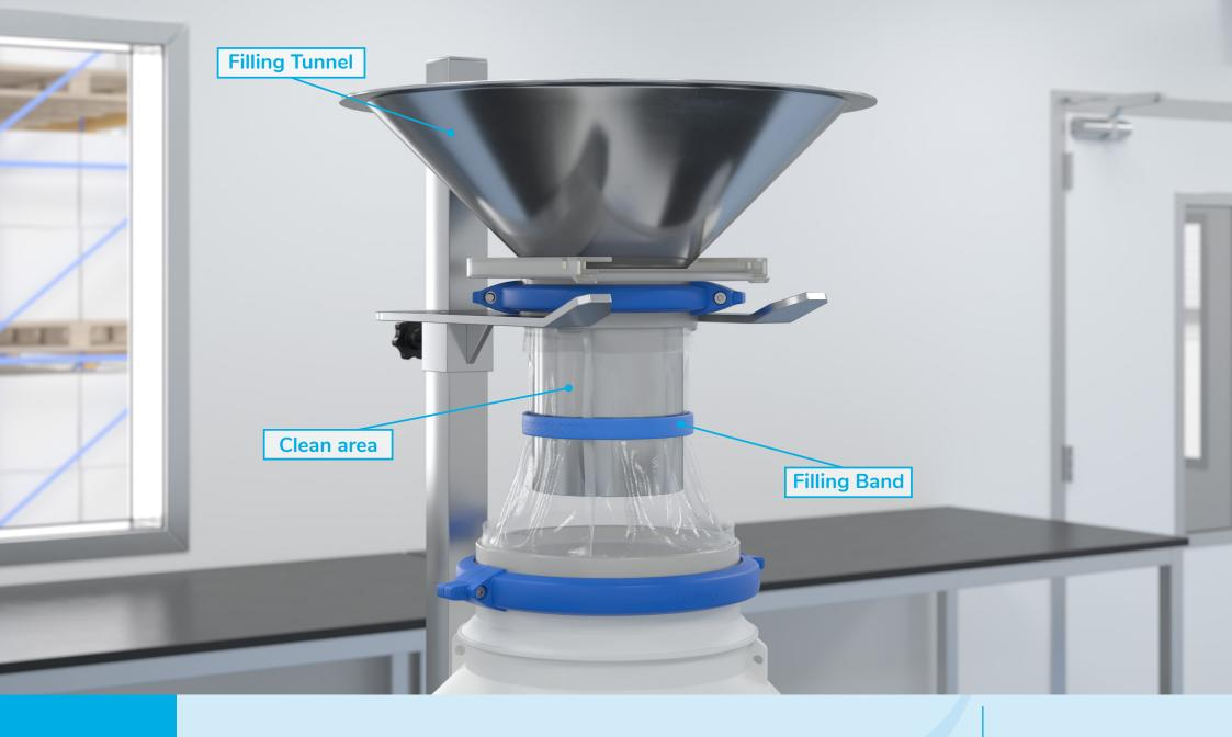
Fully insert the Filling Funnel through the Passive Body. The Filling Band must tightly wrap around the Filling Funnel and should be positioned towards the end of the Funnel Spout. This will create a "Clean Area" and prevent product from contaminating the Flexible Connector chute/bottle & Passive during the Filling Process.
