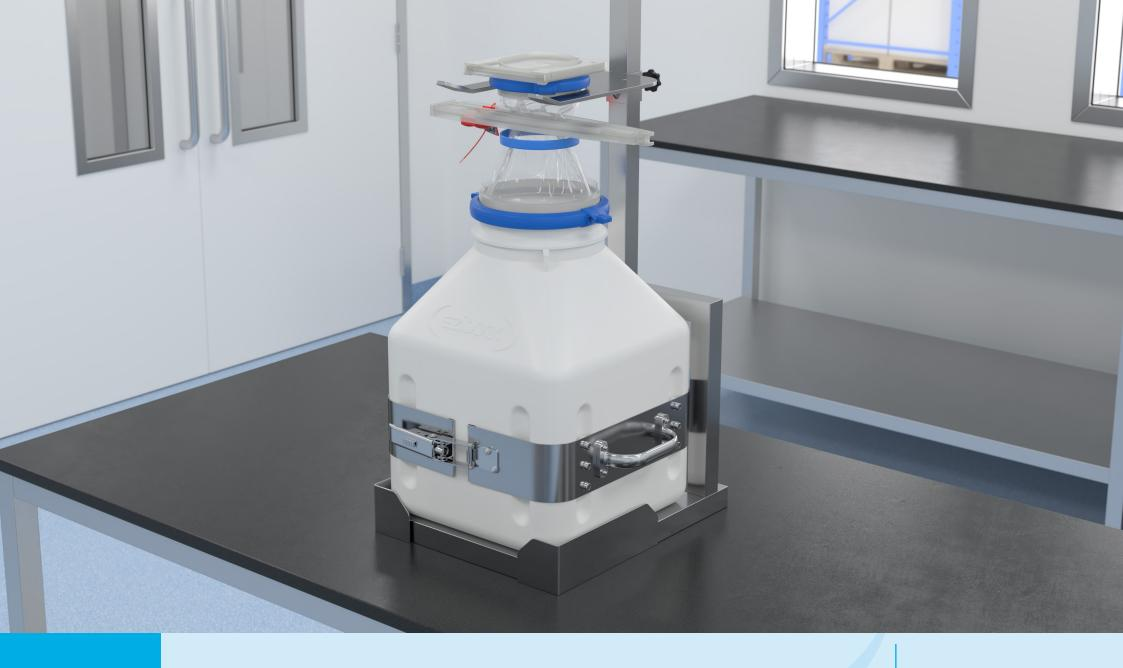
The filling procedure is now complete, and the Pharma Process bottle is now ready for discharge.
