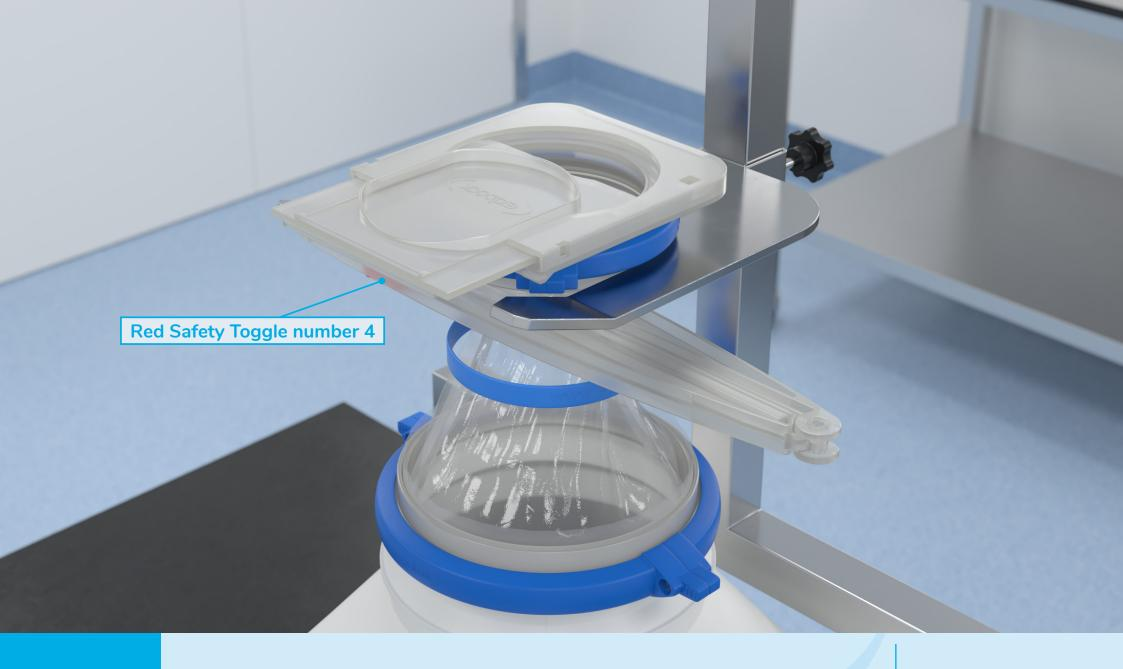
Carefully, push the two halves of the Bag Clamp together.
