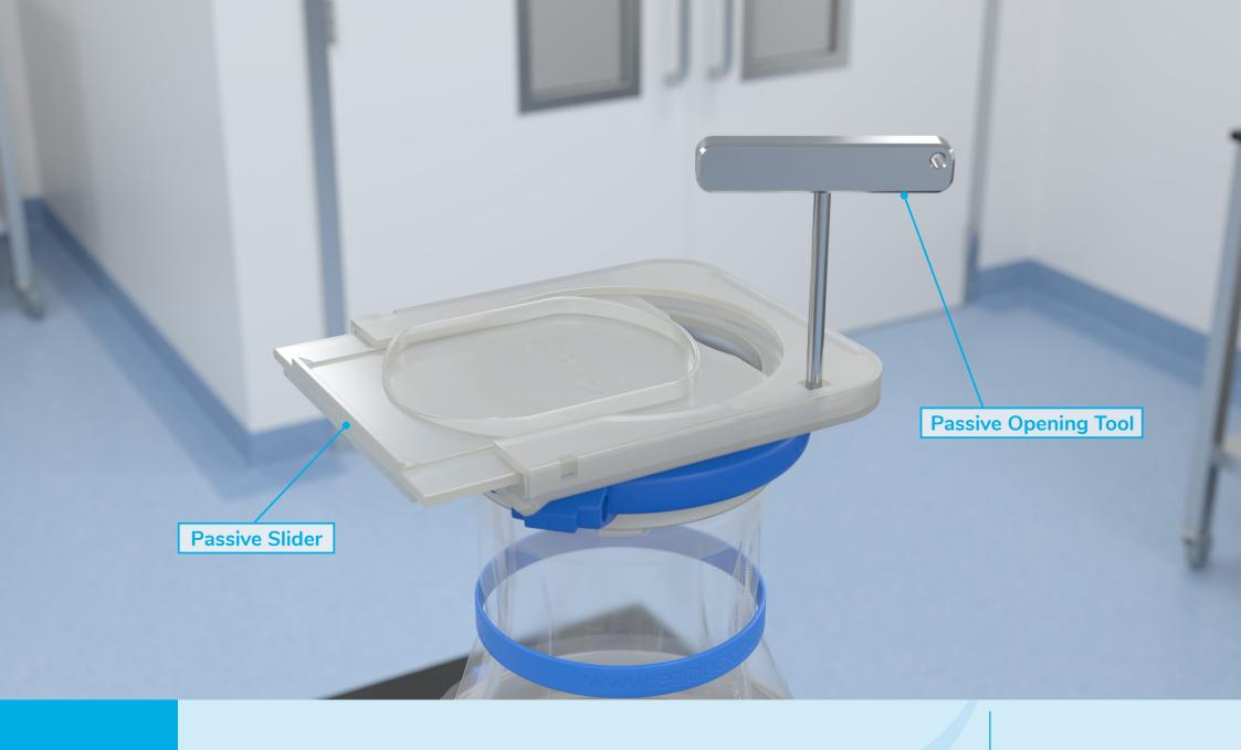
The Ezi-Flow CSV Passive has a Manual Interlock which prevents the Passive Slider from being removed. To remove the Passive Slider, simply depress the Passive Interlock Mechanism using the Passive Opening Tool.
