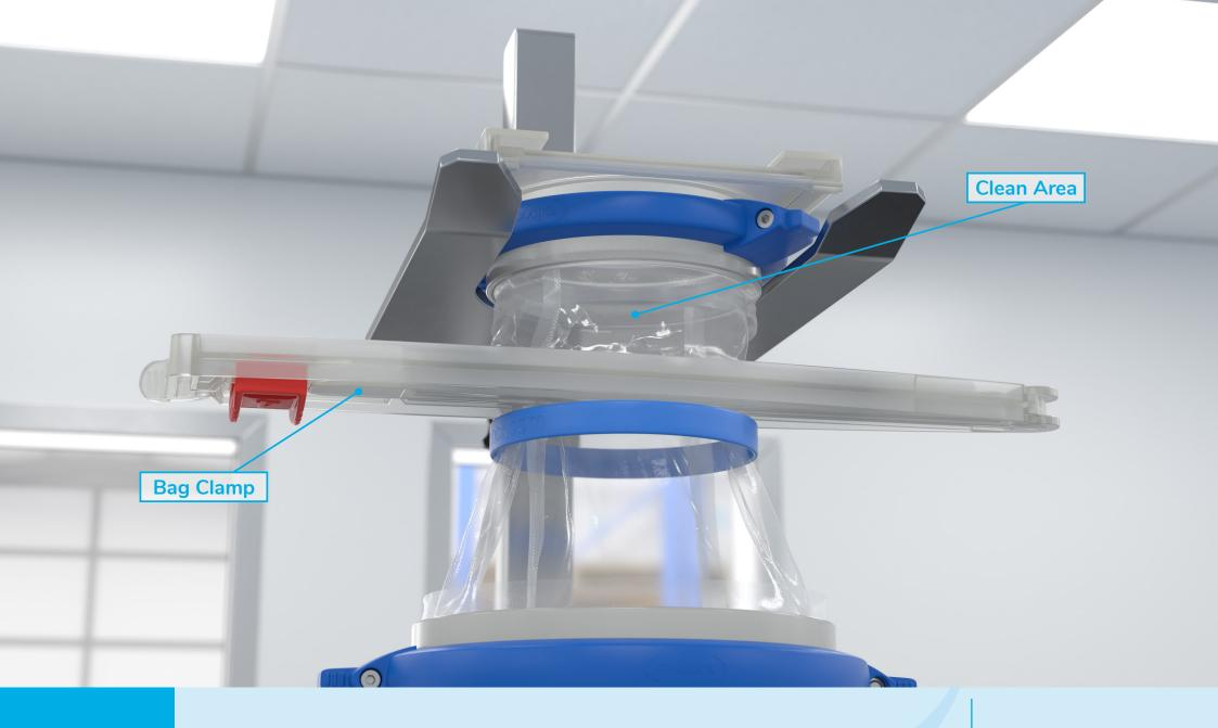
The Ezi-Grip Single Use Bag Clamp needs to be used to seal off the Flexible Connector Chute and prevent product from contaminating the Passive. Be sure to position the Bag Clamp in the "Clean Area" between the Passive and the Filling Band.
