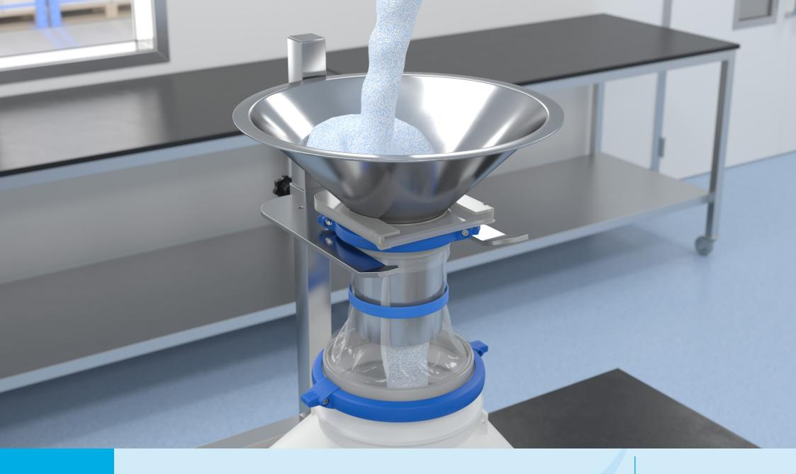
Product can now be carefully dispensed through the Filling Funnel into the bottle via the flexible connector chute.
